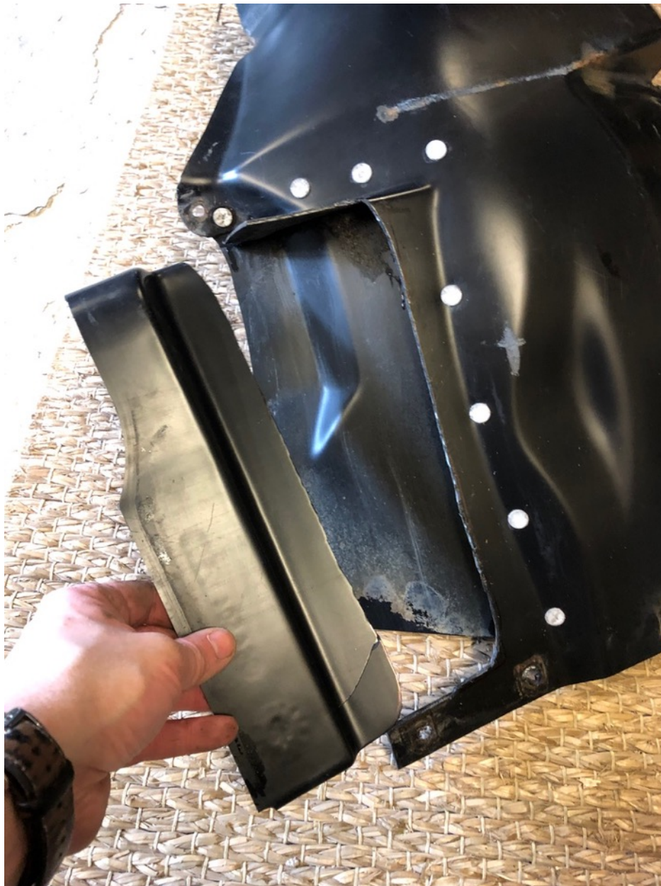
Figure 13 - Removing a section of the arch liner to clear condenser. Important to leave lower mounting holes.
