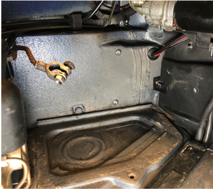
Figure 4 - Battery side showing 2 x M8 screws. Also note hole on right with grommet for wiring.
