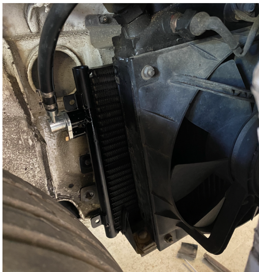
Second condenser slides in behind oil cooler.
