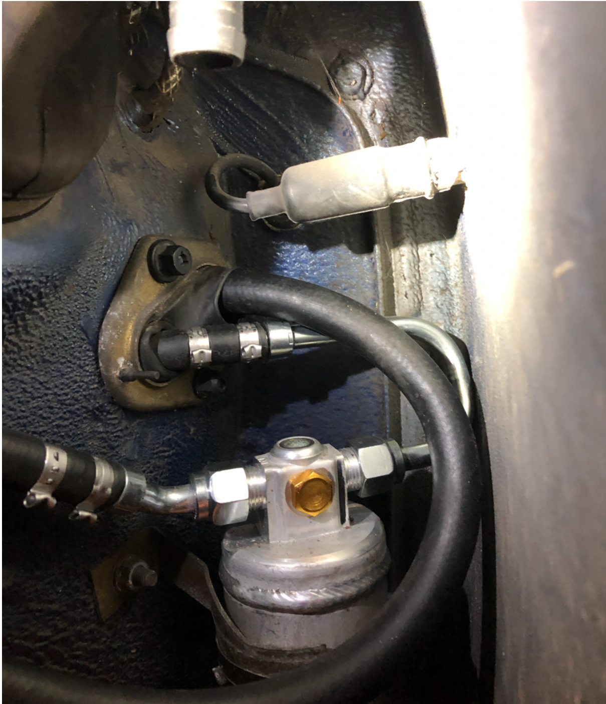
Figure 14 - Drier can be fitted in standard location.
