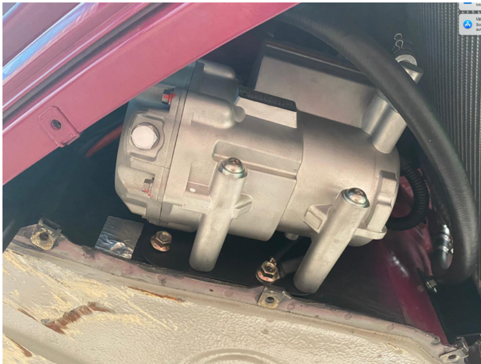
Figure 6 - View of compressor from under vehicle.
