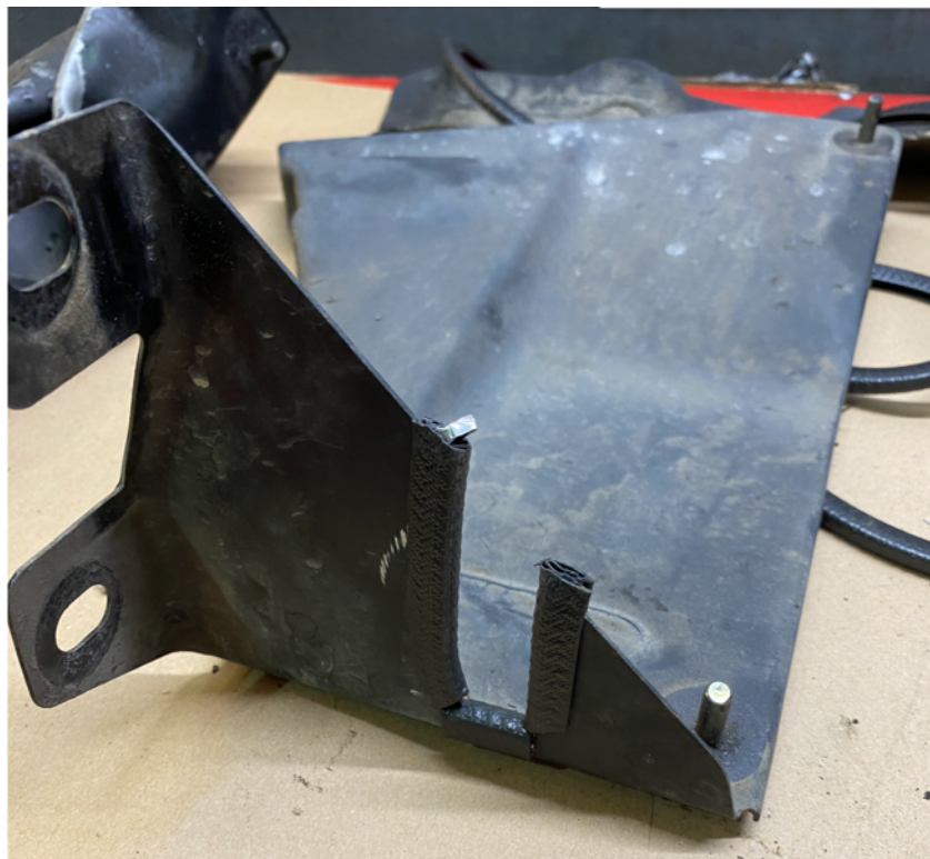
Notch cut in oil cooler support bracket.
