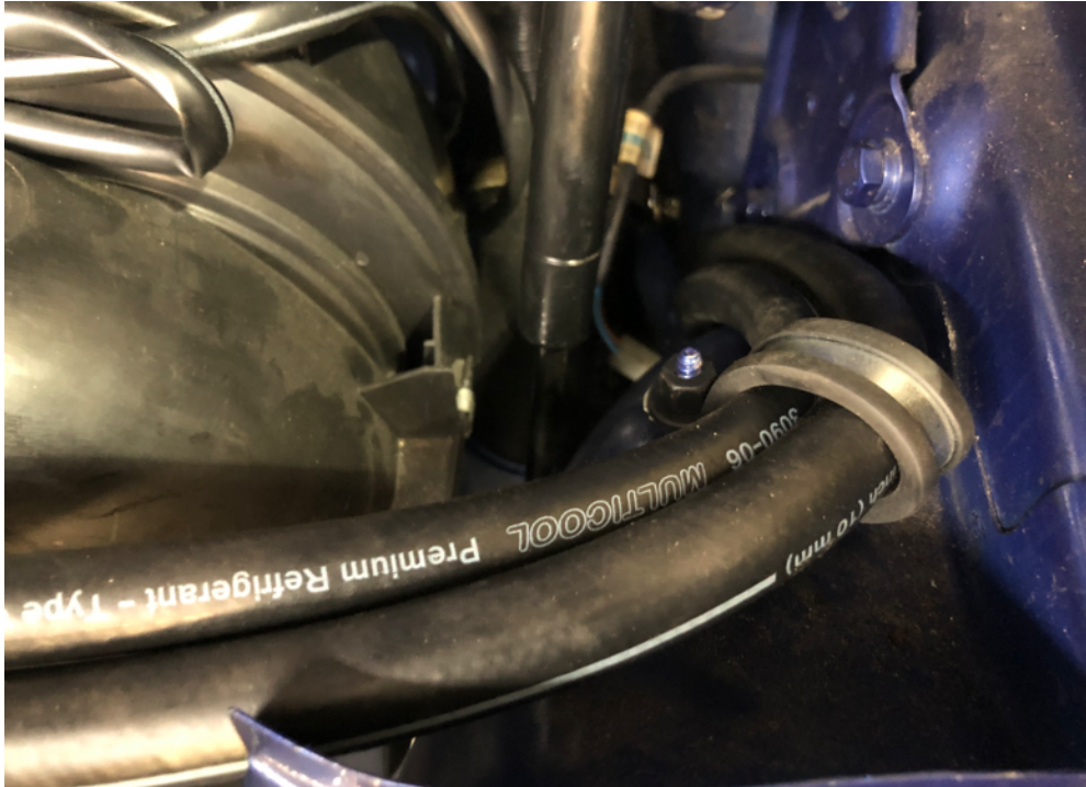
Figure 3 - Hoses secured by P-clip before going through factory inner wing hole.
