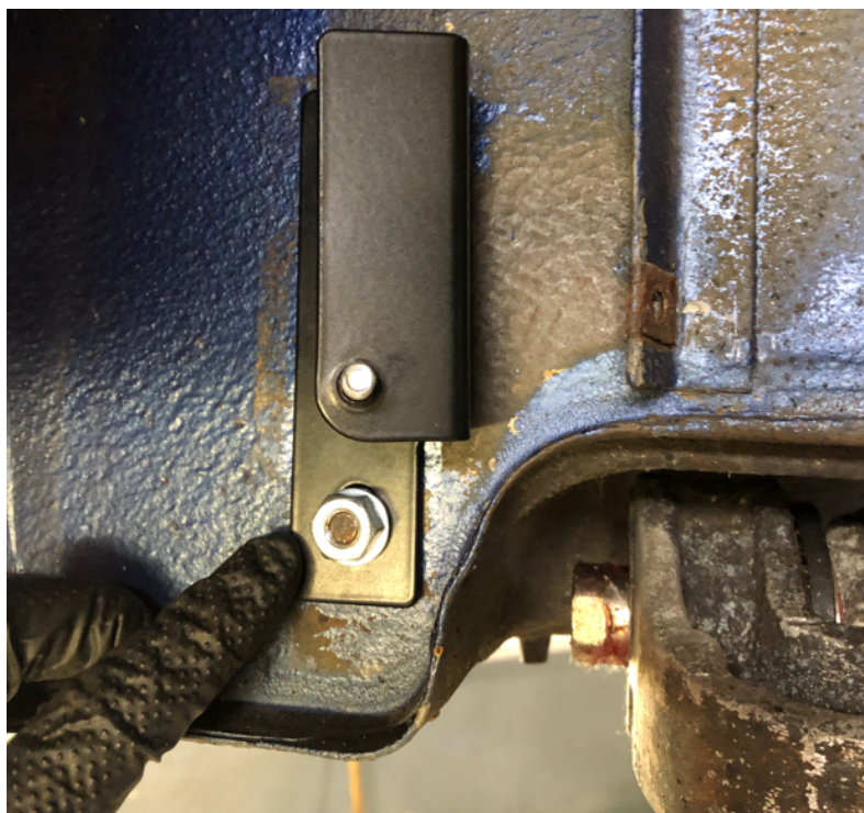
Figure 10 - Rear condenser mount bracket
