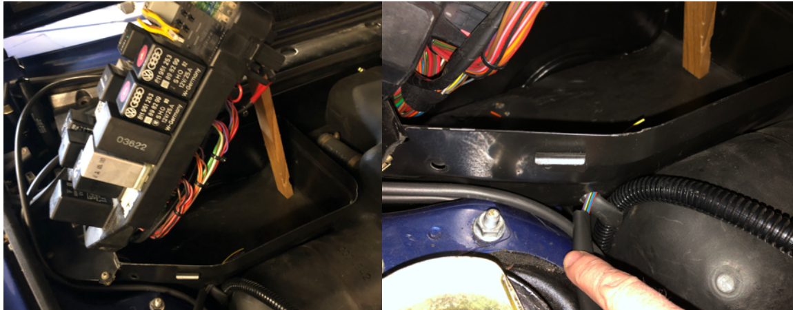
Figure 16 - Feeding Electrocooler loom into front of fusebox.
