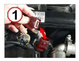
2. Click in the DCT wiring loom to the rail pressure sensor.
