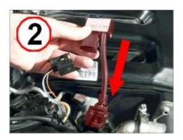
3. Re-connect the rail pressure sensor into the DCT unit
