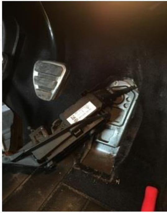
4. Disconnect connector from top of pedal unit.
