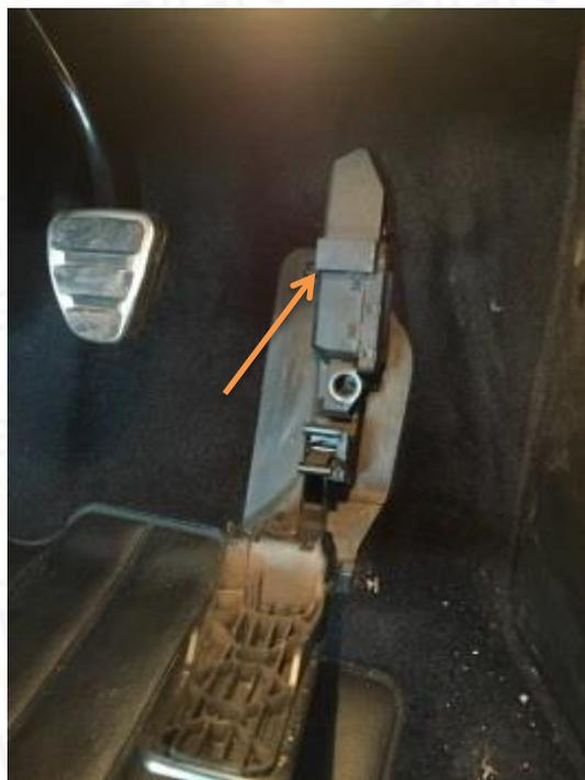
3. Lift pedal unit upwards to release from bracket.
