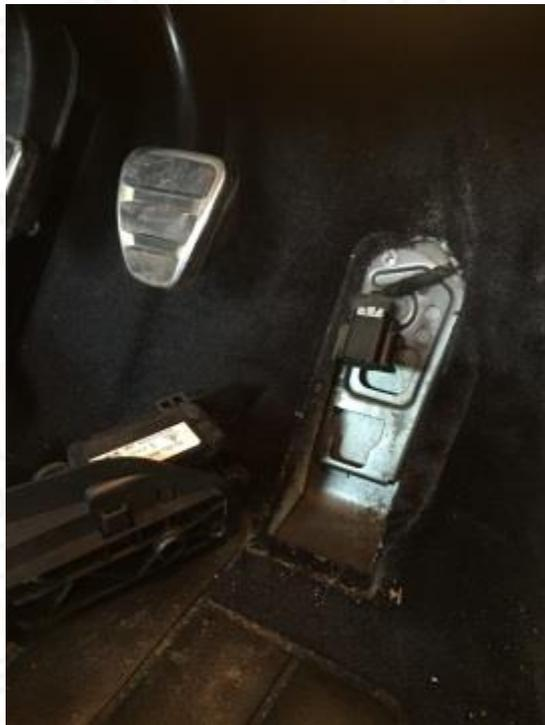
5. Pull carpet forward slightly and re-route pedal connector to appear at top of carpet.
