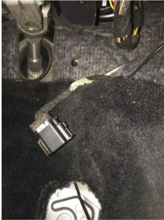
6. From I-Drive box take the piece of loom and connect to throttle pedal connector.
