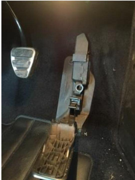
2. Pull Throttle pedal forward to reveal throttle pedal assembly.
