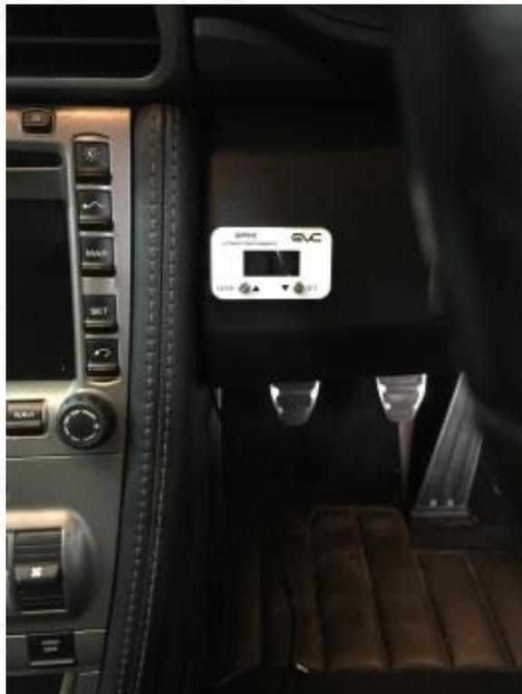
9. Run the wiring from the unit down behind between the dash and centre console so the small connector appears by the small connector of the loom next to the centre console and foot rest.
