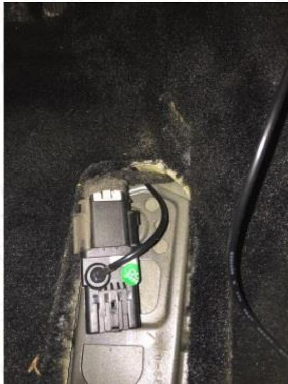
7. Run the loom behind the carpet so the small connector appears by the foot rest and centre console.
