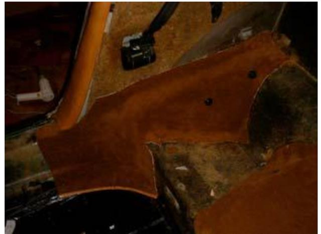
3. Carpet below side panelling (left): For '77-'86 models: same as under 2 (picture 3A). For '69-'73 models: Carpet piece over side panelling and piece over the doorframe is one large piece. As such steps 3 and 9 should be considered as one.
