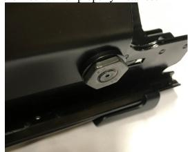
Front (left) and rear (right) bolts should sit flush with nuts if installed properly. Use loctite.
