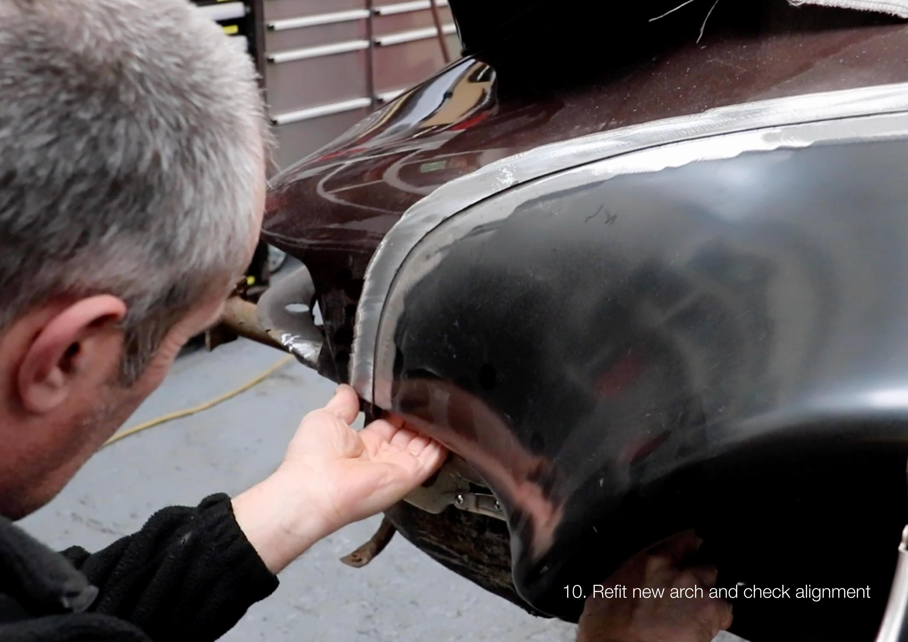
10. Refit new arch and check alignment
