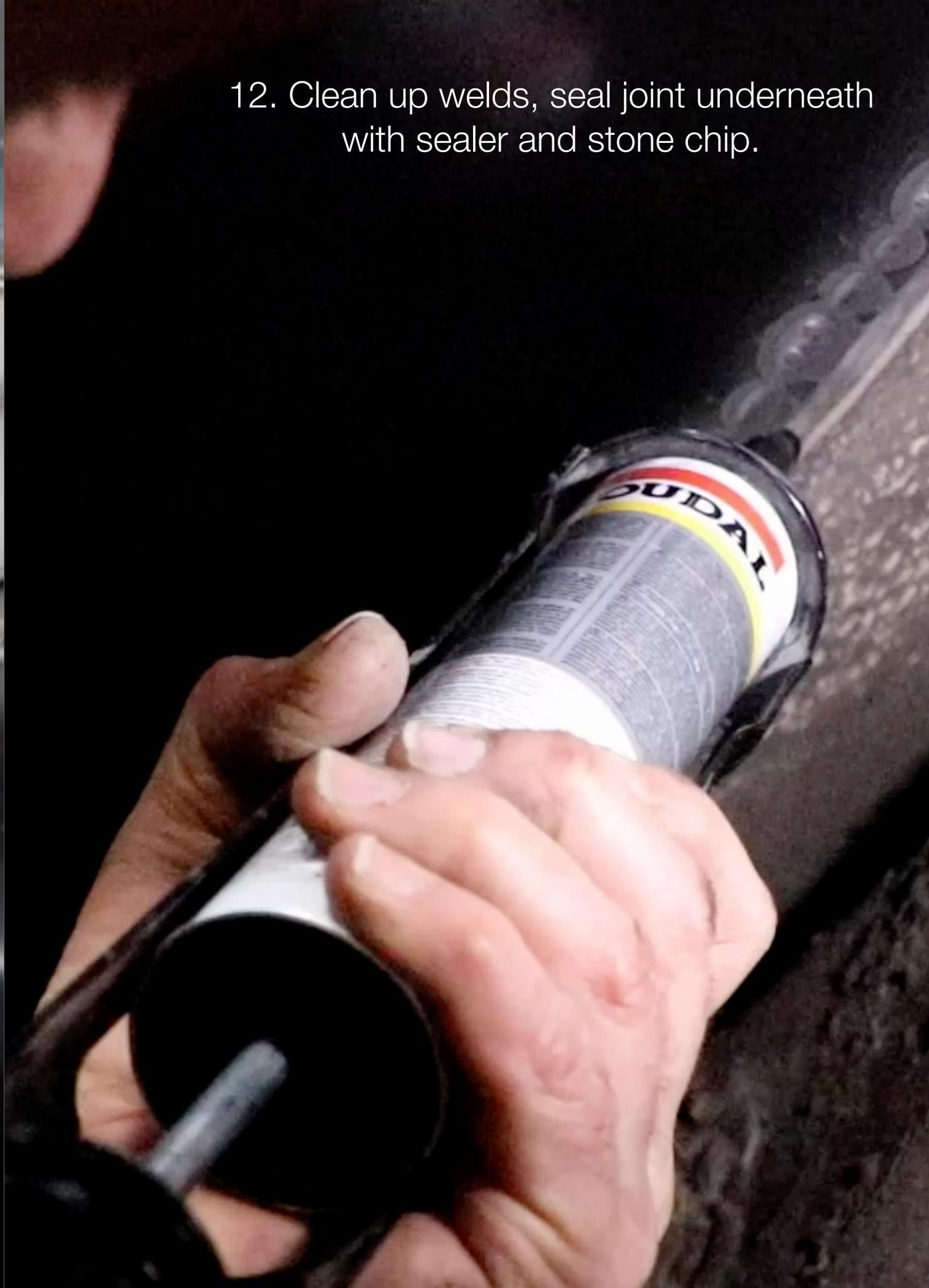
12. Clean up welds, seal joint underneath with sealer and stone chip.
