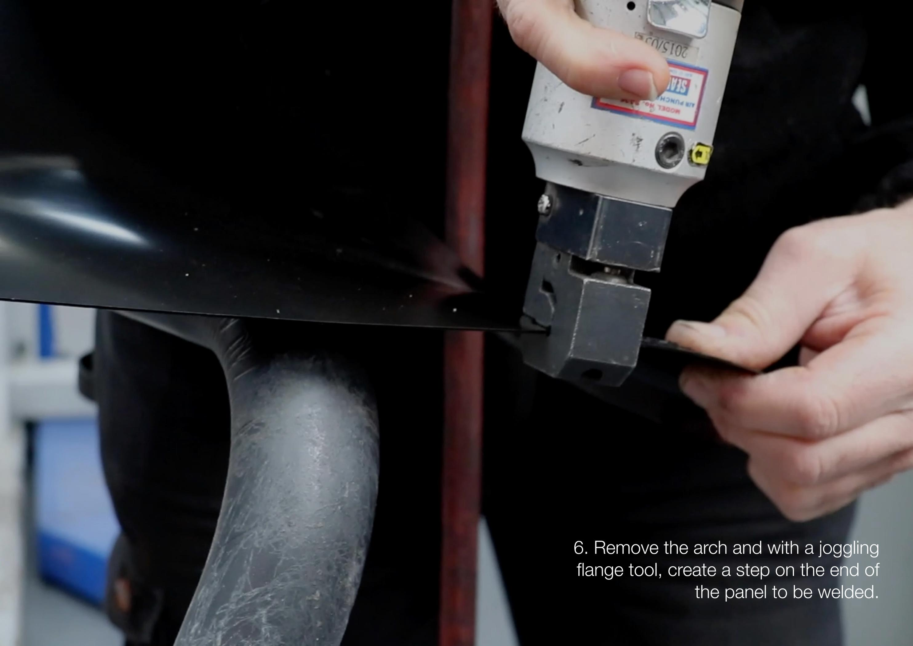
6. Remove the arch and with a joggling flange tool, create a step on the end of the panel to be welded.
