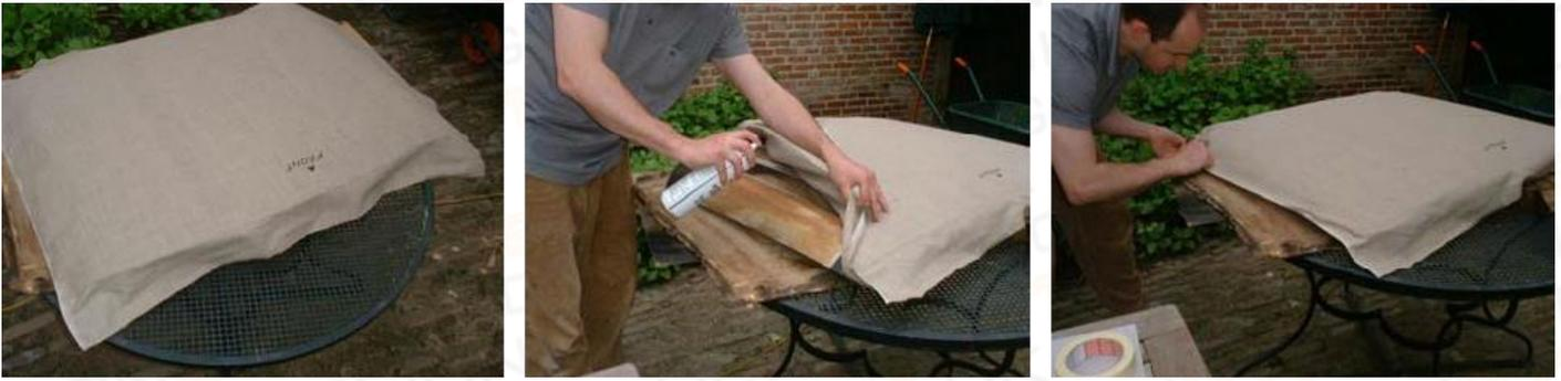
5. Apply spray glue to the inner side of the Targa top frame edges. Cut away corners at 45° (picture 5A). Flod the linen over the edge and press to fit. Use a Stanley knife to cut away excess material (picture 5B).
