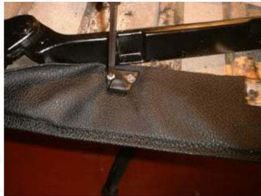
9. Now move to the back. Apply glue to the inside back edge of the frame (across the linen) between the middle Targa top clips. Proceed as under step 8.
