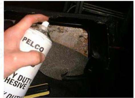
19. You are now ready to instal the headlining at the back. Remove the Targa top clips and proceed as under stop 17.
