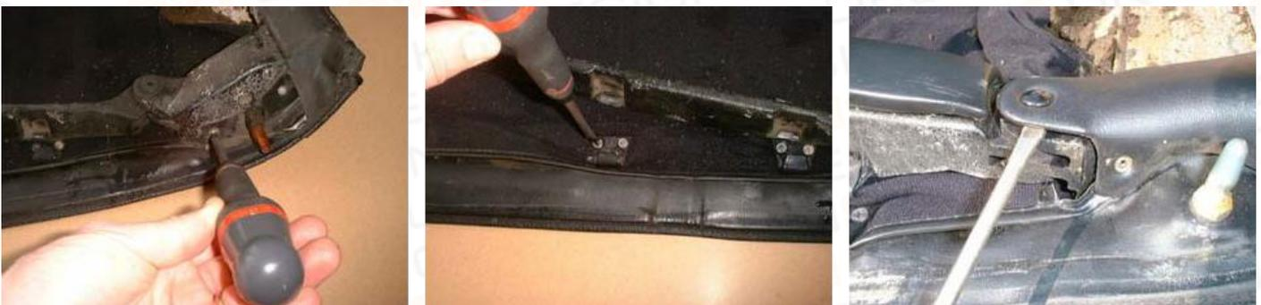
2. Remove the rubber seals on both sides of your top by taking out the screws in the rubber apertures (picture 2A). Now remove the 2 steel guides left and right (picture 2B). Use a metric spanner (M13) to remove the top guide pins (picture 2C). Your roof skin can now be removed.
