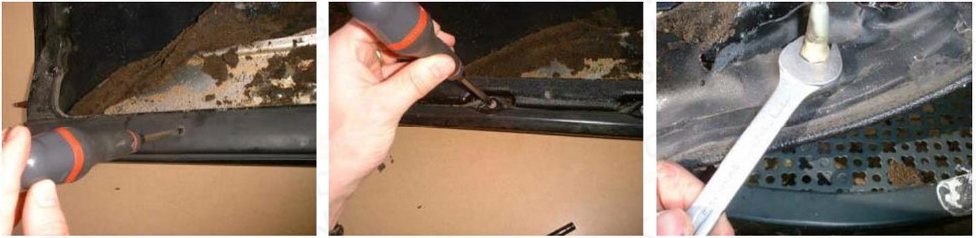
3. Once your roof skin is taken off, the linen and padding can be removed. Your top is now fully dismantled. Inspect the frame for proper operation. In particular, pay attention to the condition and snugness of the tension bands (under thumb on picture) when the tension bars are in their extended position. Correct, clean and paint as required. Do not throw away your old top pieces. 'Reading' your old top may help to install new ones to perfection.
