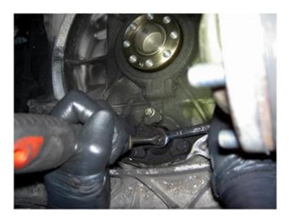
Remove the three flange support bolts.
