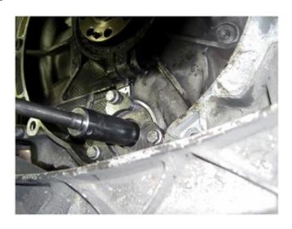
If you need to replace the Rear Main Seal (RMS) this is the time. Use a strong metal pick to pull out the damaged seal and install the new one in place. Follow the RMS' installation procedures (depending on the manufacturer).
