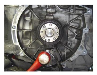
a bead of thread lock onto the three clean flange bolts
