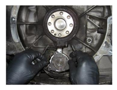
Using a flat screwdriver turn it Counter Clockwise (ccw) to get the first two or three threads of the center shaft exposed
