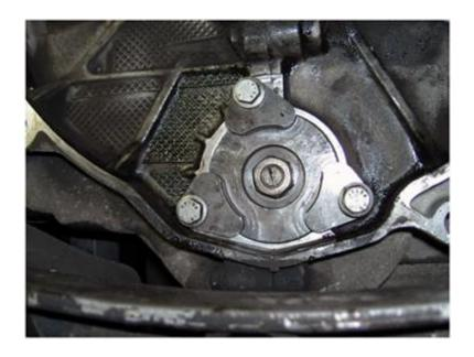
After the flange is in place, tighten the center nut. You may have to hold the center shaft from rotating using a flat screwdriver just the opposite of when it was loosened
