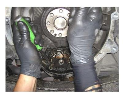
With the flange out, remove the bearing's retaining c-clip.
