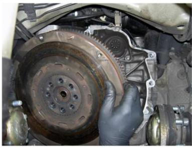
At this time, inspect the Rear Main seal for sings of leaks. If it is leaking it would be wise to replace it after installing the Eternal IMS Fix.
