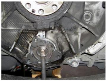
Once the first couple of threads are out, insert the center nut and tighten by hand.
