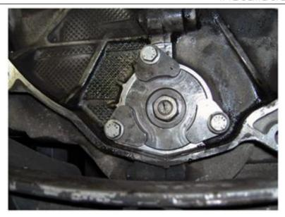
After the flange is in place, tighten the center nut. You may have to hold the center shaft from rotating using a flat screwdriver just the opposite of when it was loosened
