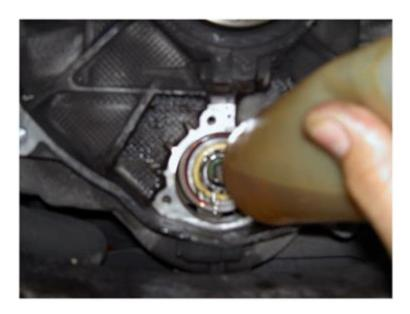
Smear a bit of grease onto the new flange's O-ring to allow for an easier installation
