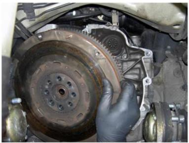
At this time, inspect the Rear Main seal for sings of leaks. If it is leaking it would be wise to replace it after installing the Eternal IMS Fix.
