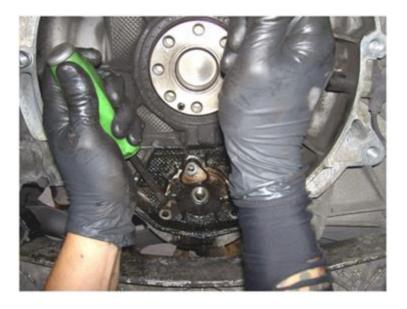
With the flange out, remove the bearing's retaining c-clip.
