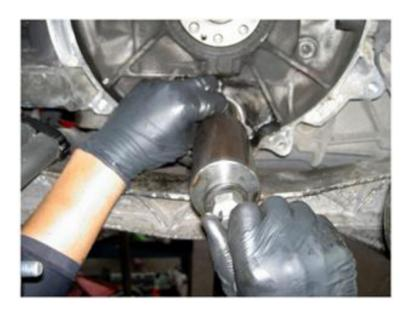
... and thread the center bolt onto the IMS bearing shaft. Tighten it by hand. Tighten the tool's center nut by hand all the way down making sure that the IMS Removal Tool is completely seated at the base of the engine block.
