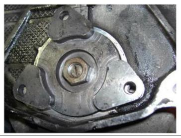
With the new flange centered, carefully tap it in with a brass or rubber mallet, being careful not to hit the bearing's center shaft
