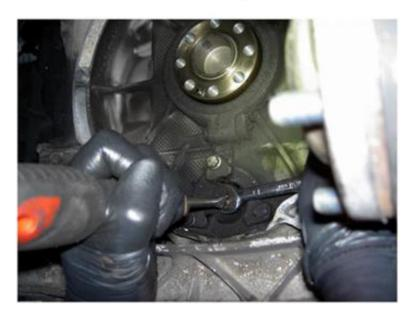
Remove the three flange support bolts.
