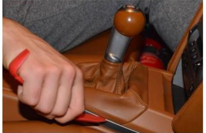
**Step 2:** For cars with integrated boot/knob, use a razor blade to cut the factory boot all the way around base of the factory knob leaving boot as long as possible. Remove factory knob from the boot. For cars without integrated boot/knob, skip to step 3.
