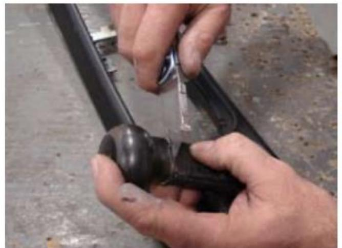
**Step 4:** Pull the knob out of the boot until the O-ring will not allow you to pull any further. Re-install shift boot/knob assembly. Set desired height of the shift knob and tighten the set screws at the base of the knob.
