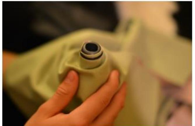
**Step 3:** Turn the boot inside out and insert the knob until the base of the knob is even with the base of the boot. Install rubber O-ring over the boot and align with the groove in the knob.
