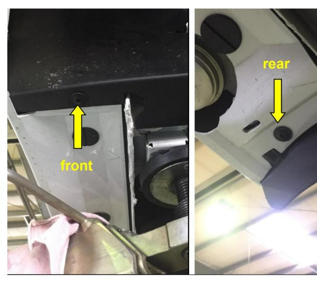
7. Remove all large plastic clips at the bottom of the door sill by twisting them (90°).
