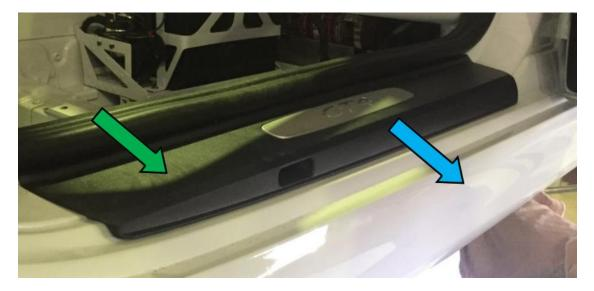
4. Remove the four black plastic spreading rivets with a suitable tool, we recommend a plastic trim removal tool.
