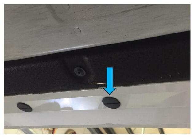
8. On the areas marked red, the door sill is fixed in holding strips by me ans of snap-in lugs. Carefully pull the door sill out of the retaining tabs.
