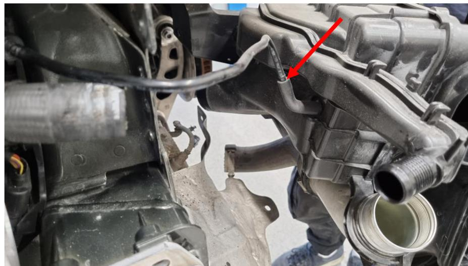
**29.** Remove the air filter box from the plastic cage.
