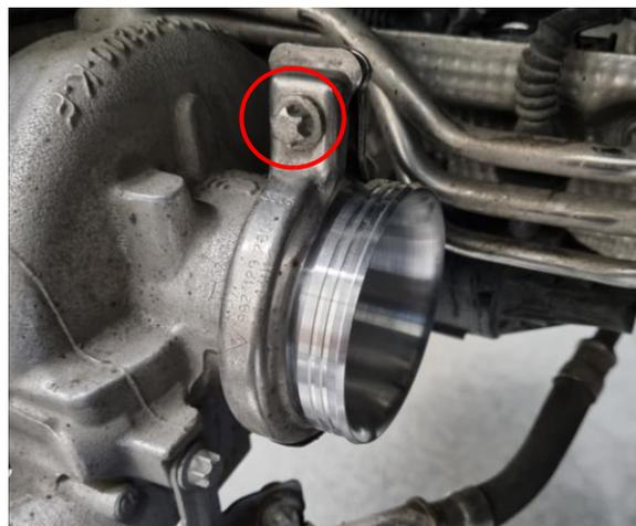
**36.** Install the inlet hose. Tighten the included 60-80mm / 9mm wide hose clamp loosely so the hose still can rotate on its connection.
