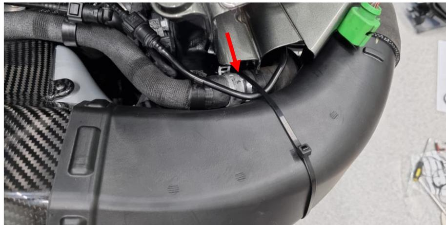
**42.** Reinstall the plastic air filter housing cage. Align the carbon fiber air filter housing so you have a few millimeters of clearance around the air filter housing. You may need to loosen the M6 Screw/nut for the large round bracket to adjust the rotation of the airbox. Finally install the included M6 washer and M6 Nut and then tighten all hose clamps. Reinstall all other parts in reverse order.
