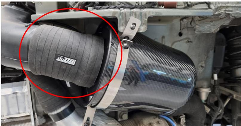
**41.** Strap the BOV hose and vacuum line (right side only) with the included zip-tie around fresh air duct. Make sure the zip-tie is placed where the aluminum joiner is.
