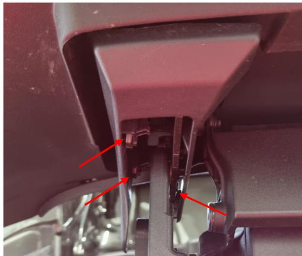
3. Remove the brake light from the spoiler. Gently push a short flat screwdriver into the holes in the two marked positions and pry the light loose. Disconnect the cable and separate the cable and grommet from the spoiler.
