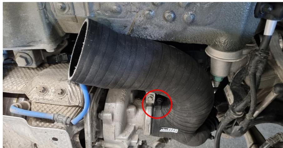
**37.** On the right side you need to disconnect the lower clips for the breather valve hose.
