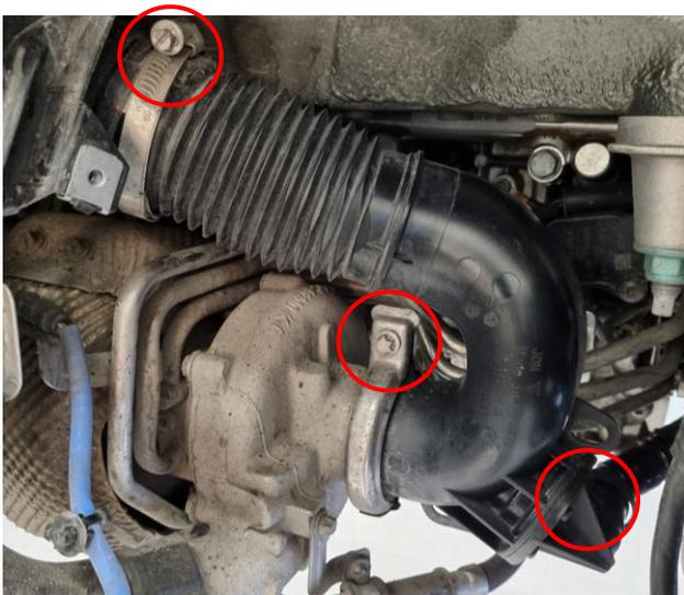
**24.** Loosen the turbo outlet hose clamp.
