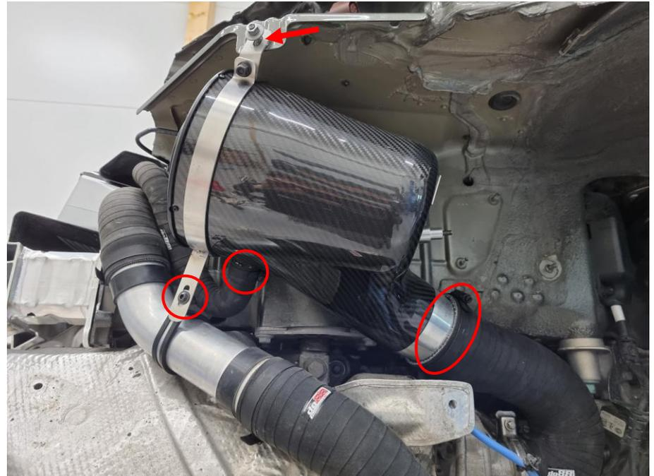
**40.** Install the plastic fresh air duct to the included square shaped silicone hose at the airbox inlet. Fasten with a hose clamp on the air box side only.
