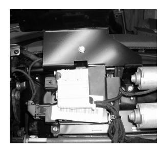
Step 10. Insert the plug removed in step 3.
