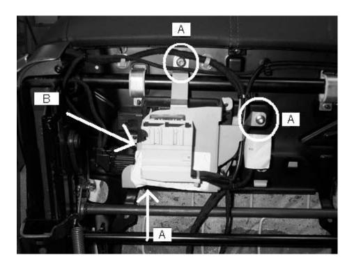
Step 5. Tilt the module to access the mounting hole. Use one of the removed self tapping screws to thread this hole.( At Location B)
