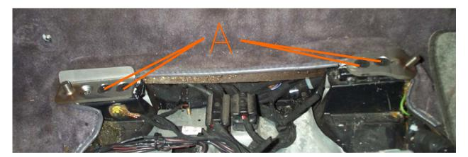
Not shown: Check the center to center distance on the studs. The side to side distance between the studs should be 16". Adjust if necessary.
